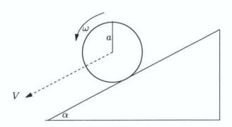
The point on the circumference of the disc that is instantaneously in contact with the plane is instantaneously at rest, because of the no-slip condition. This means that V and  $\omega$  are related by
