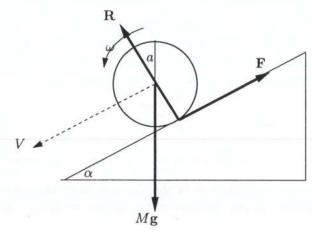
The forces acting are gravity, friction and normal reaction. Thus
