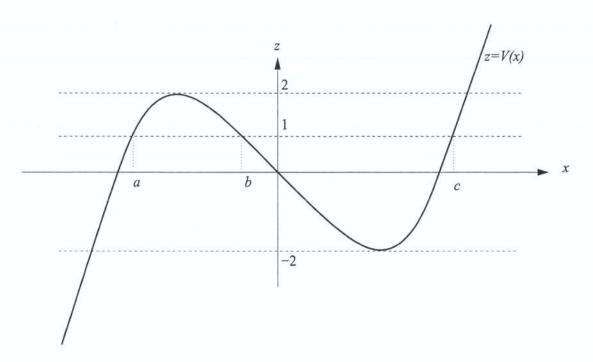
From the diagram, we can see the following possibilities (there are many others), depending on the initial conditions. For convenience, the initial conditions are given in terms of  $x_0$  and E, rather than  $x_0$  and  $\dot{x}_0$ .
