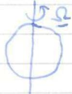
Note that  $\rho \Omega \times (\Omega \times \mathbf{x})$  is a constant (intive) and conservative body force. So the centrifugal force just adds to the hydrostatic pressure, so globally, the sea surface, for example, is not spherical.
