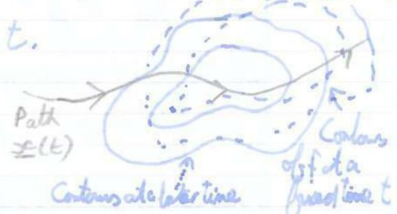
If  $\underline{x}(t)$  is the Lagrangian path followed by a fluid particle then  $\dot{\underline{x}}(t) = \underline{u}$ , the local fluid velocity. We write  $\frac{df}{dt} = \frac{Df}{Dt}$  for the time derivative along a path (trajectory) of a fluid particle.
