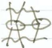
An Euler-Cycle is a "walk" round the graph using each edge exactly once, and returning to the start (initial vertex).
